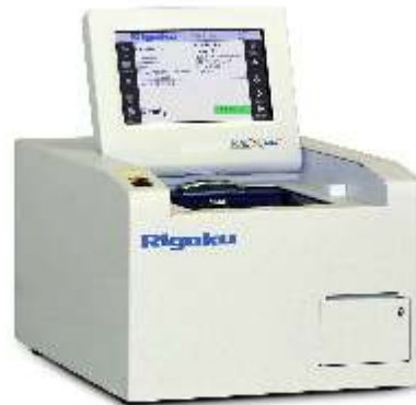
Rigaku NEX QC+ high-resolution benchtop EDXRF analyzer
